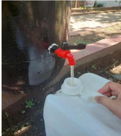
Gambar 5.1 Proses pengambilan air lindi sisa endapan biogas
